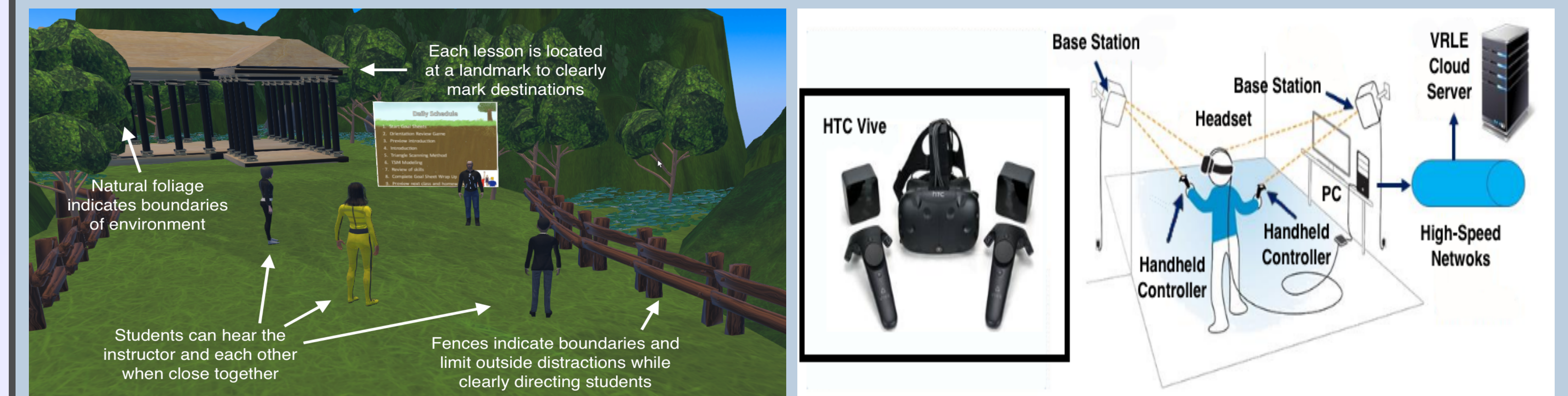
Figure 2: Major components of the experimental testbed setup for the usability study with HTC Vive and VRLE cloud server (left); Overlook of a iSocial standards compliant VRLE module demonstration with slide show and avatars of an instructor and three students (right)
